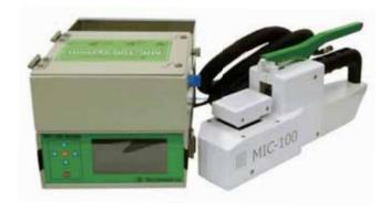
MIC-100 is a very unique system to measure photosynthesis rates at high speed by focusing measurement tools on the photosynthesis ability of plant leaves.
